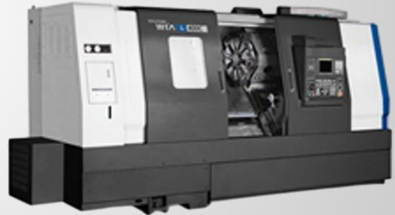
Hyundai-Wia L400C Max. Turn Ø630mm Max. Length 1170mm Max. Weight 500Kg
